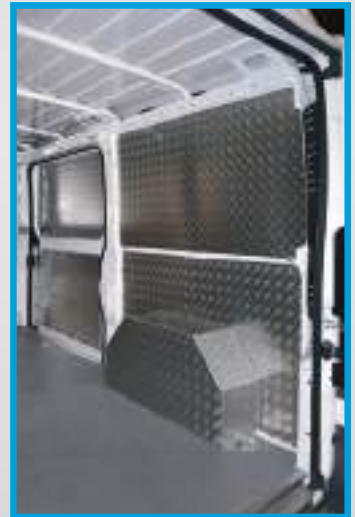
Ducato/Boxer/Jumper 2006/Movano 2022: Floor liner in marble-look beech plywood, bodywork and bulkhead liners in aluminium tread plate, wheel arch covers in aluminised steel sheet and aluminium tread plate
