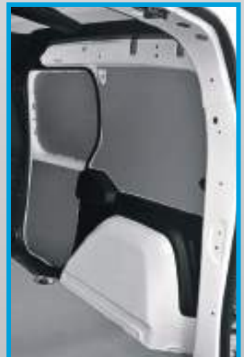
Ducato/Boxer/Jumper 2006/Movano 2022: Floor liner in marble-look beech plywood, bodywork and bulkhead liners in aluminium tread plate, wheel arch covers in aluminised steel sheet and aluminium tread plate
