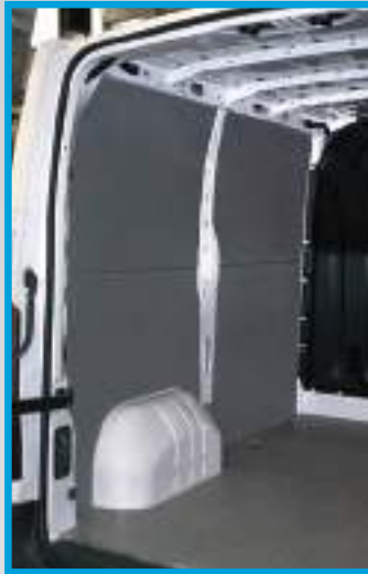
Master/Movano/NV400 2010: Floor liner in marble-look beech plywood, bodywork liners in grey prepainted steel sheet
