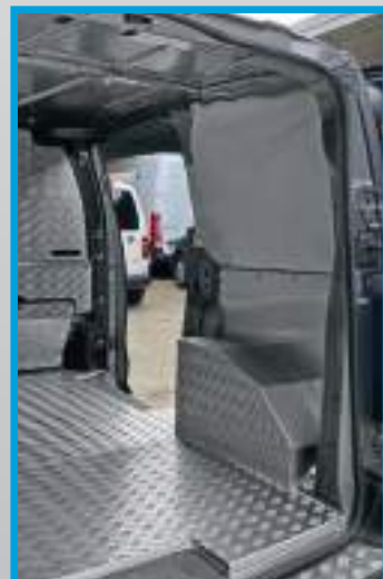
Expert/Jumpy/Proace 2016/Vivaro 2019/Scudo 2022 L2 H1: Double-layer floor liner in 9 mm birch plywood and aluminium tread plate, bodywork liners in aluminium, bulkhead liner in aluminium tread plate, wheel arch liners in aluminised steel and aluminium tread plate
