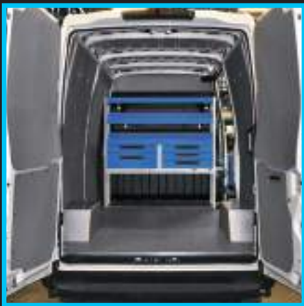
Iveco Daily: racking on the bulkhead only.
