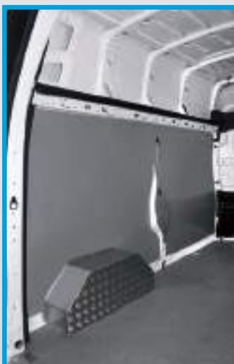
Vivaro/Trafic 2014/Talento 2016/NV300 H1: Floor liner in marble-look beech plywood, bodywork liners in grey prepainted steel sheet, wheel arch covers in aluminised steel sheet and aluminium tread plate
