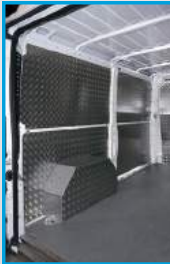
Ducato/Boxer/Jumper 2006/Movano 2022: Floor liner in marble-look beech plywood, bodywork and bulkhead liners in aluminium tread plate, wheel arch covers in aluminised steel sheet and aluminium tread plate
