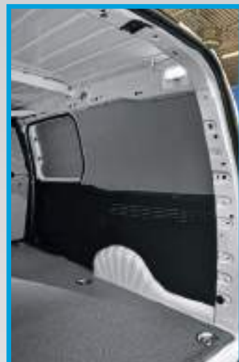
Berlingo/Partner/Combo/Proace City 2018 L2: Floor and bulkhead liners in marble-look birch plywood, bodywork liners in grey prepainted steel sheet
