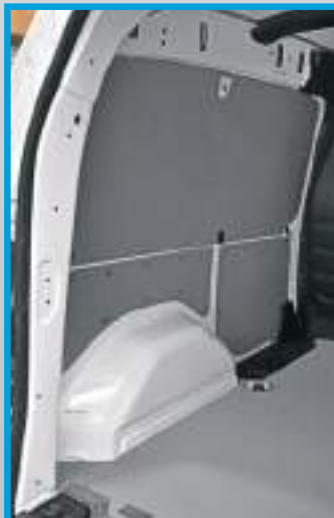
Ducato/Boxer/Jumper 2006/Movano 2022: Floor liner in marble-look beech plywood, bodywork and bulkhead liners in aluminium tread plate, wheel arch covers in aluminised steel sheet and aluminium tread plate
